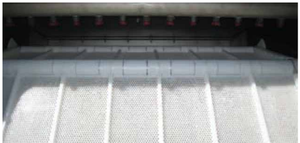
Patented mesh panels eliminate the problem of hairpinning and blinding
