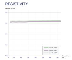
All data are typical values. Resistivity, TOC, metals rinse performance measured after 12 hrs. at 30 BV/h with  $\geq$ 17.5 M $\Omega$ -cm rinse water. The special properties of the OvivUP resins can only be fully guaranteed if the technology and processes used correspond to Ovivo recommended operating conditions.
