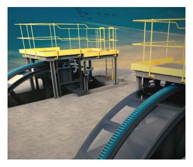
**New Debris / Eel Collection hopper** – the existing debris collection hopper has been replaced with a new unit which has two separate sections; the first section is designing to capture the eels & water from the elevators and gently flush the eels, via a flood lauder trough, back to the river. The second stage captures the weed/trash backwashed off by the high pressure backwash and is discharged into a debris collection
