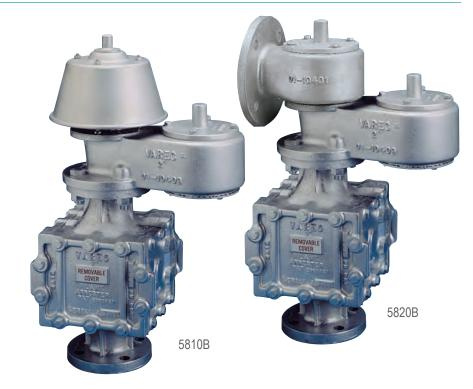
The flame arrester is designed to stop the propagation of a flame by absorbing and dissipating heat through the surface area of the bank sheets. Heat is absorbed as ignited gas attempts to pass through the small passages within the bank assembly. This action lowers the temperature of the gas below its ignition point and quenches the flame.
