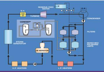
Typical configuration of a high pressure boiler and associated condensate polishing plant, and CONESEP® external regeneration technology
