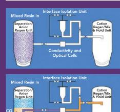
Exhausted, mixed resin is transferred to the resin separation/ anion regeneration vessel. A small amount of mixed resin, isolated during the previous regeneration, is added from the resin isolation pot. The resins are backwashed and air scoured to remove particulates.
