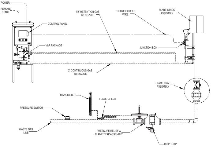
Figure 01: 244W - Typical Installation
