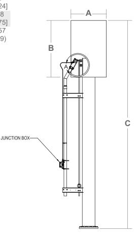
NOTE: Standard height of the flare stack is 15 feet to meet the minimum requirement per ANSI / CSA B149.6. The actual flare tip must be determined based on radiant heat at ground level. Consult factory for assistance. Stack dimensions are the same for all the options available with the 244WS or 244WL.
