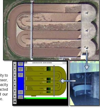
Ovivo's process engineers recommended simply replacing the existing aerators with more powerful and efficient 200 HP Excell®Aerator II's and to operate them using VFDs and Ovivo's aeration and nutrient control system. After a thorough evaluation of all options, the Ovivo recommendation was selected as the most cost effective and efficient alternative.
