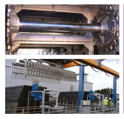
The robust design of the Brackett Green® Traveling Band Screen is highlighted by the robust headshaft construction of these screens awaiting dispatch.
