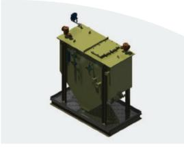
The OVIVO Sep equipment uses coalescing plate packs that induces small oil droplets to combine into larger, more easily separable droplets. The distributor plate spreads the flow evenly over the width and height of the plate packs. The individual plate packs are sloped to a 45° or 60° angle to minimize the possibility of sludge fouling.
