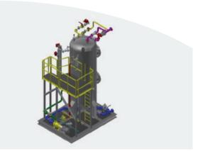
Pressurized water passing through the eductor creates a vacuum at the gas suction port, whereby the gas is induced from the head space in the IGF Vessel and induced into the water stream. This is essentially a closed loop with very low gas consumption such that make-up gas requirements are 0.25 to 0.5 scf per barrel of produced water treated.
