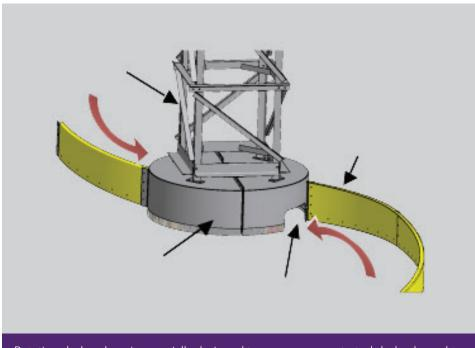
Rotating sludge drum is especially designed to remove concentrated sludge brought by the spiral blades to center of the tank
