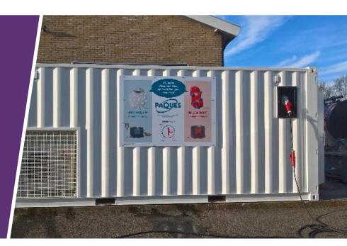
The pilot plant is proposed to confirm treatability of the subject wastewater stream containing Ammonia and Phosphorus. The unit can be operated under different conditions and in different configurations. It is containerized and complete with automation and controls ensuring reliable results. Biomass behavior can be analyzed and different loading rates can be applied so that relevant operating data for scale-up is produced.
